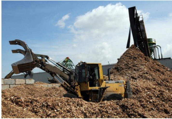
The Lafarge cement plant (top) now burns 15 per cent process-engineered fuel, which consists mainly of wood waste ground up at Urban Woodwaste Recyclers (above).
